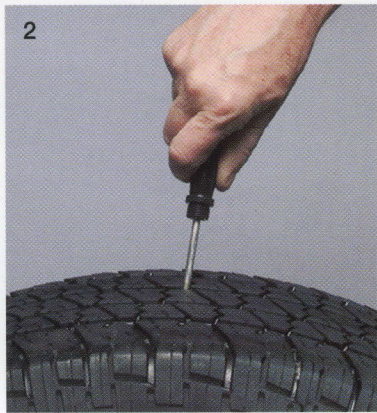
2 Use probe tool to inspect damage
