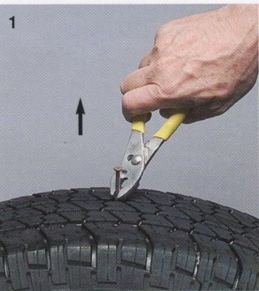
1 Locate puncture and remove damaging item
