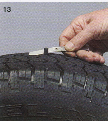
13 Inflate tire to full pressure and then trim stem at tread level
